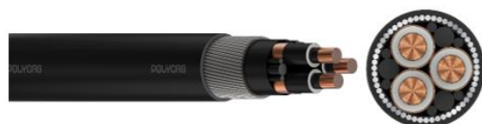
POLYCAB MV CU BS 6622 3.8/6.6 KV - Medium Voltage Armoured Cable, 3.8/6.6 (7.2) KV AC
