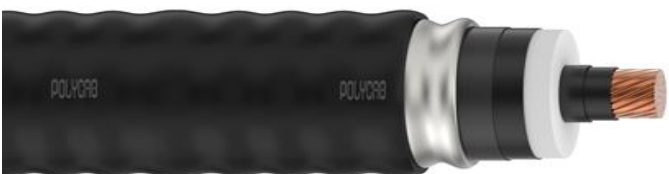
POLYCAB HV AL.COR IEC 60840 38/66 kV (72.5 kV) - Copper Conductor
