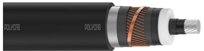
POLYCAB HV CS+PAL IEC 60840 127/220 kV (245 kV) - Aluminium Conductor
